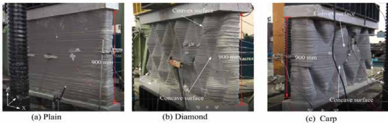
Fig.8: a) Shape and Dimension of the Tested Walls b) Testing of 3D Printed Walls with different Geometries [5]
