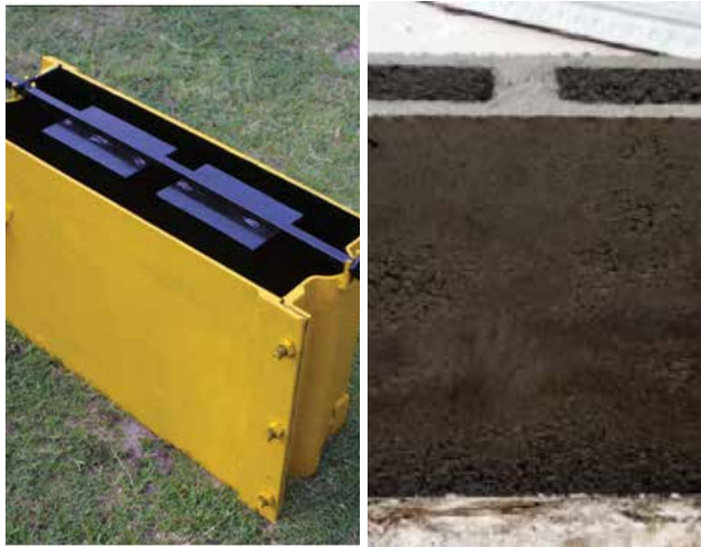
Fig. 7: Full Size Steel Mould and Hollow Block Specimen (150 x 450 x 300 mm)
