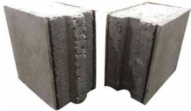
Fig. 4: Lightweight Sandwich Panel with Tongue and Groove Provisions
