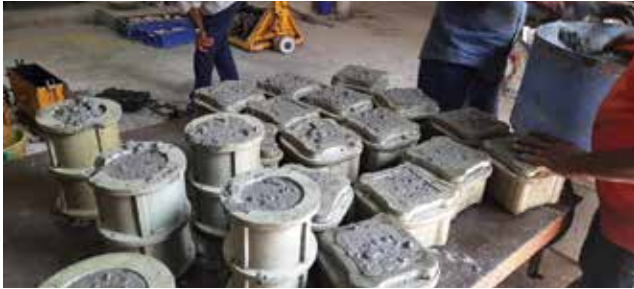
Fig. 5: Casting of Various Specimens
