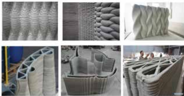
Fig.5: Complex Shapes and Textures of 3D Printed Walls [2, 3, 4]
