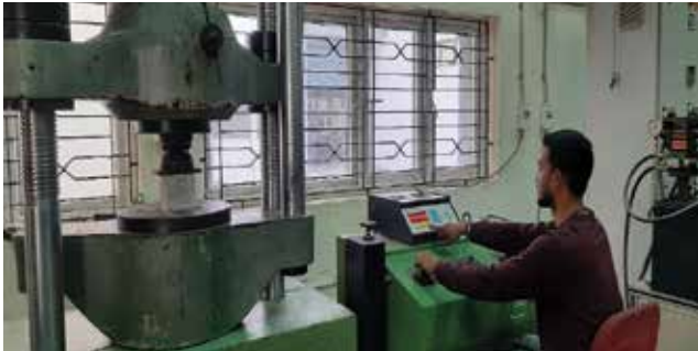
Fig. 6: Compression Test of Cube Specimen
