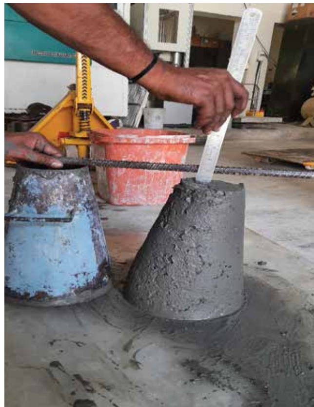
Fig. 4: Slump Test of Fresh Concrete
