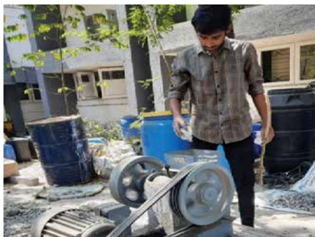
Fig. 3: View of Jaw Crusher
