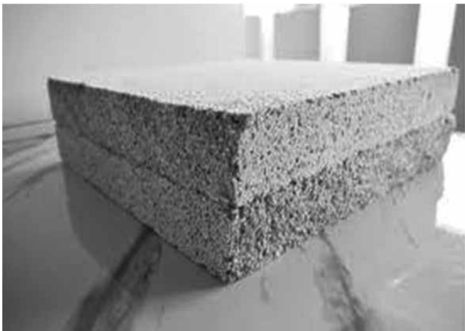
Fig. 2: Aerogels insulation board used as facade in roofing
