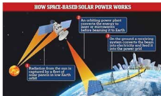
Fig. 2: Beaming solar energy from space to earth
