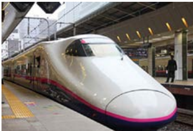
Kingfisher's Beak Shaped Nose of Bullet Train to reduce noise
