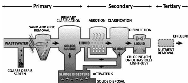
**Fig. 1: Treatment of Liquid Waste**
