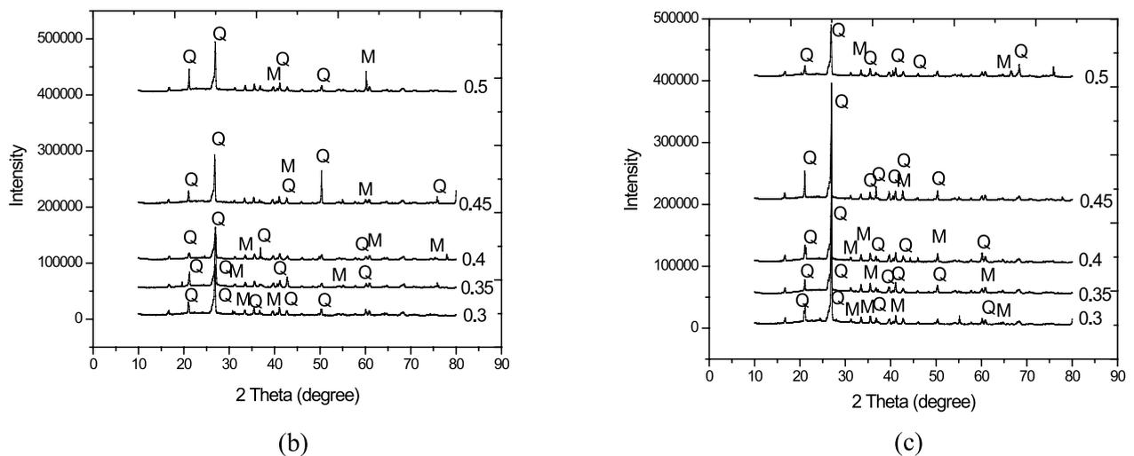
**Fig. 2: XRD analysis of (a) Fly-ash and Geopolymer (b) 7 days' curing (c) 14 days' curing**
