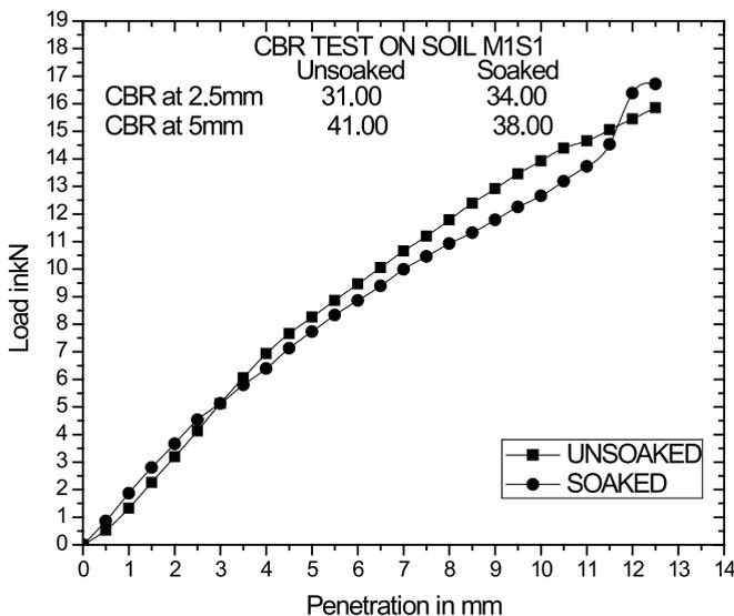
**Fig 15: CBR curve of M1S1**
