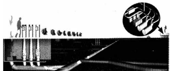
**Fig. 4: Pneumatic Waste Collection System**
