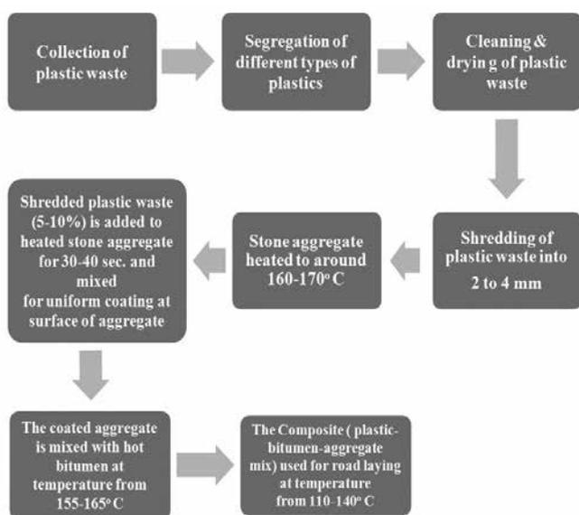
**Fig. 3: Process Flow Diagram of Plastic Coated Bitumen Mix**
