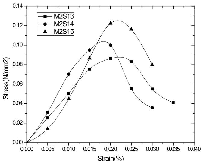
**Fig. 11: Unconfined Compressive Strength Curves of Different Soil Sample with Different Percentage of Cement.**
