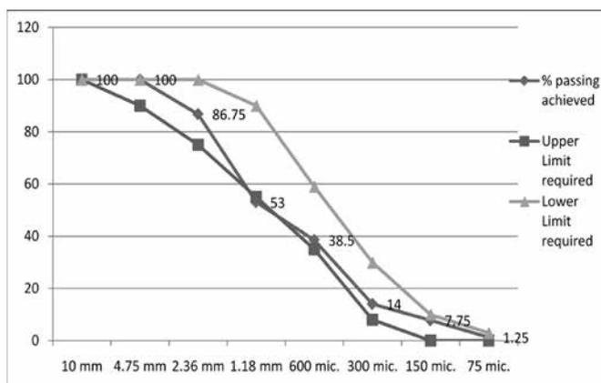
**Fig. 5. Particle Size Sieve Analysis (Coarse Sand) (a) Fresh Fine Aggregate**
