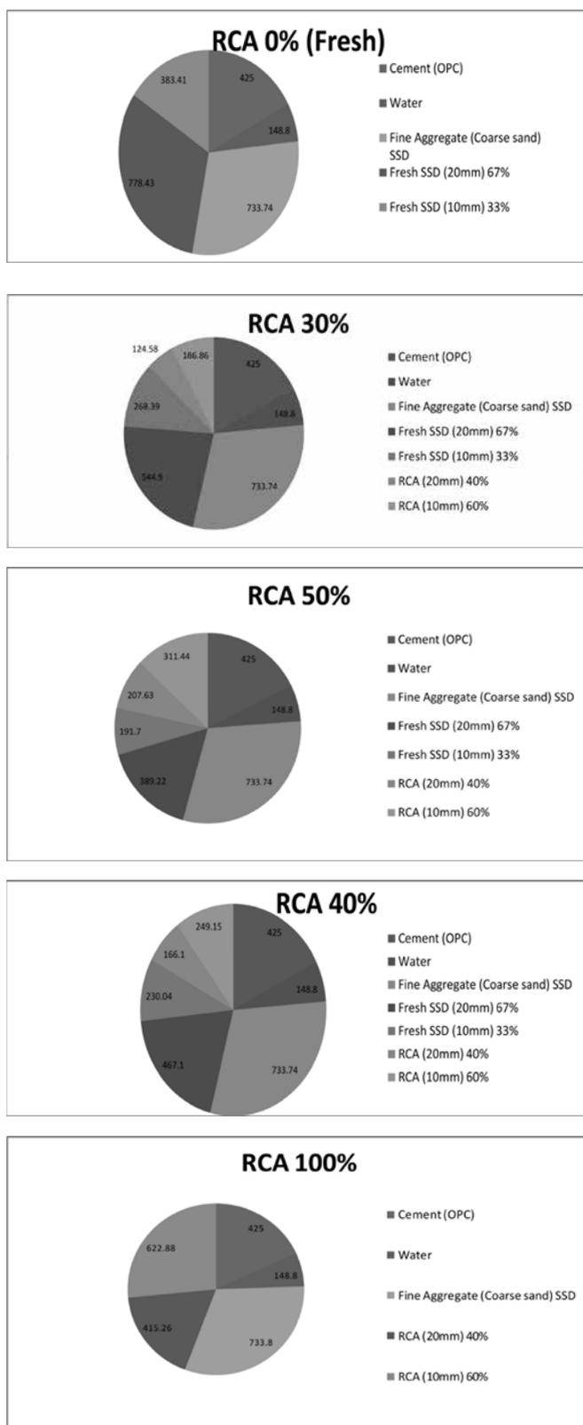
**Fig. 7 Various Trial Mixes of M 40 Pavement Quality Concrete using Different Percentages of RCA (SSD : Saturated Surface Dry Condition)**
