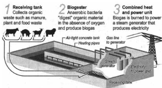
**Fig. 2: Producing Electricity from Methane**
