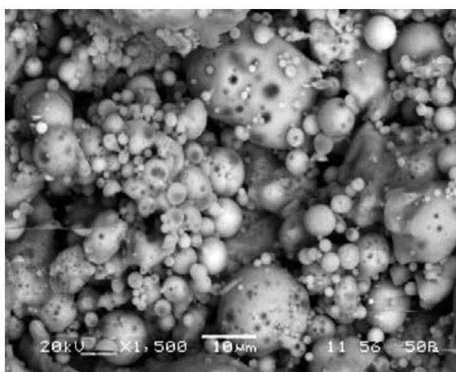
**Fig. 6: Scanning Electron Micrograph of Fly-ash**
