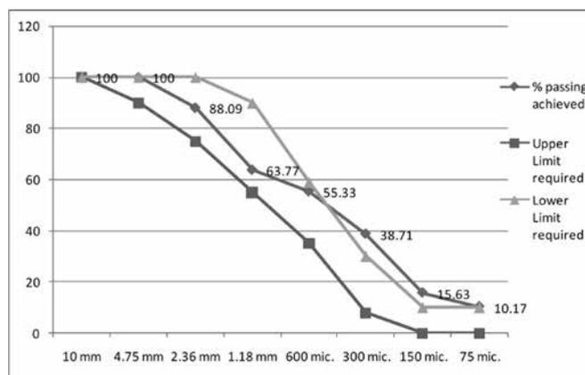
**Fig. 5. Particle Size Sieve Analysis (Coarse Sand) (b) Fine Aggregate (RCA)**
