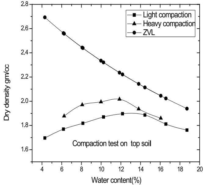
**Fig. 10: Compaction Test on Top soil**
