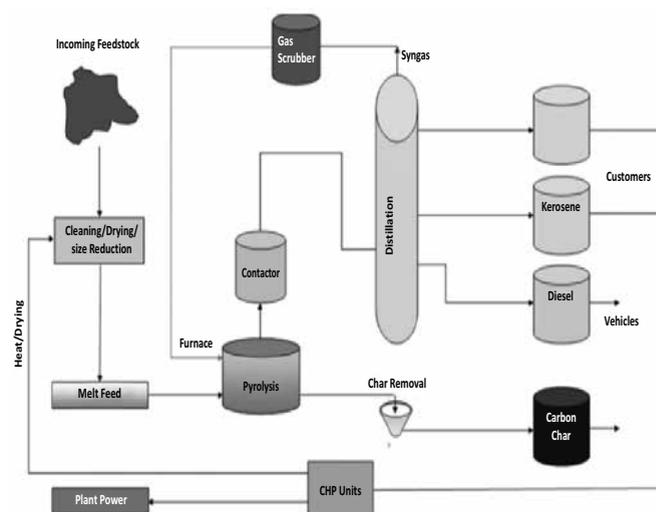
**Fig. 6 Waste Plastic Pyrolysis Process System**
