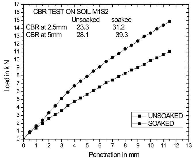
**Fig 16 : CBR curve of M1S2**
