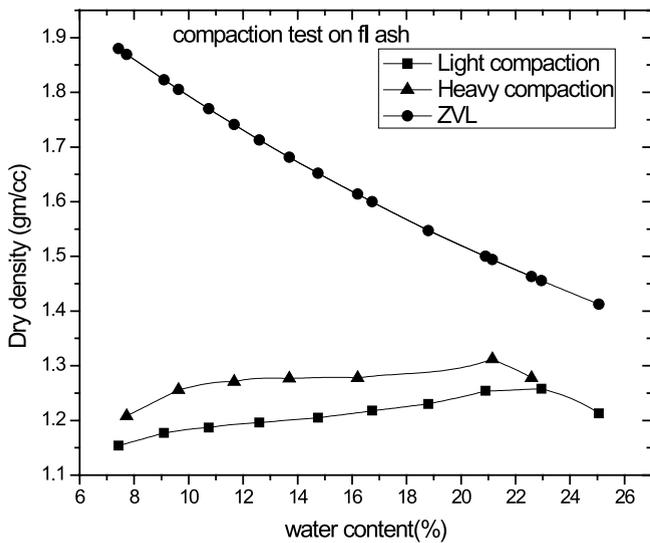
**Fig. 8: Compaction Test on Fly-ash**
