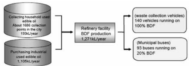
**Fig. 5: BDF Production and Uses in Kyoto City**
