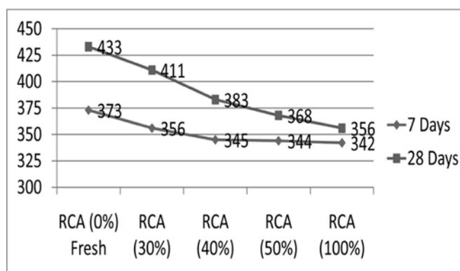
**Fig.8 : Comparison of compressive strength of Cement Concrete M-40 (PQC)**
