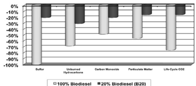
Fig. 1. Comparison of Emission between B100 and B20 Fuel
