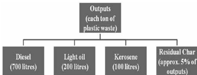
**Fig. 7: Outputs of Pyrolysis Process**
