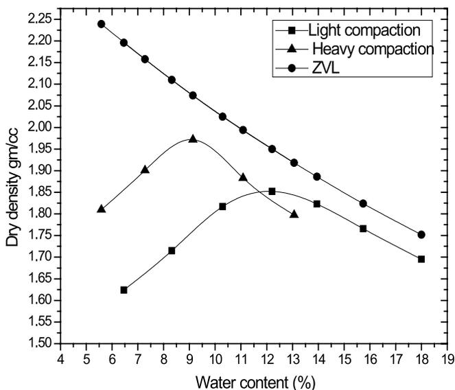
**Fig. 9: Compaction Test on Shale**
