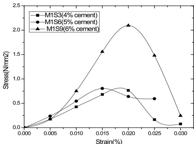
**Fig. 12: Unconfined Compressive Strength Different Soil Sample with Different Percentage of Cement.**
