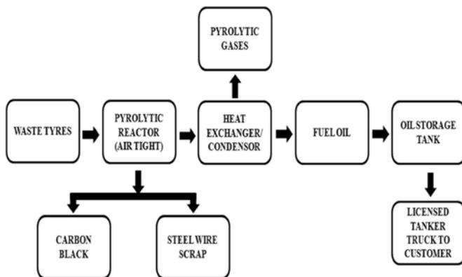
**Fig. 6: Pyrolysis Plant Process**
