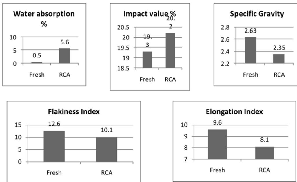
**Fig. 4 Comparison of RCA with Fresh Aggregates**
