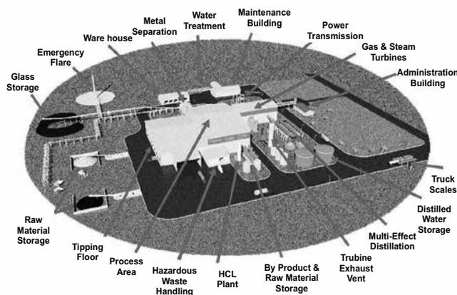
**Fig. 3: The Multi Activity Waste to Energy Complex** (Source: Energy Planet)
