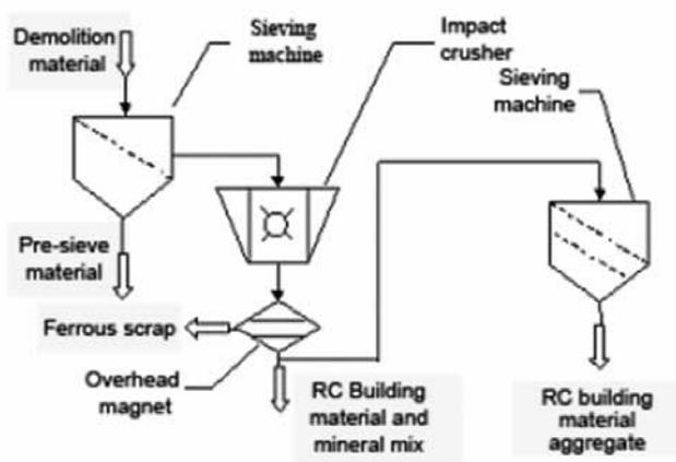
**Fig. 2: General Recycling Process**
