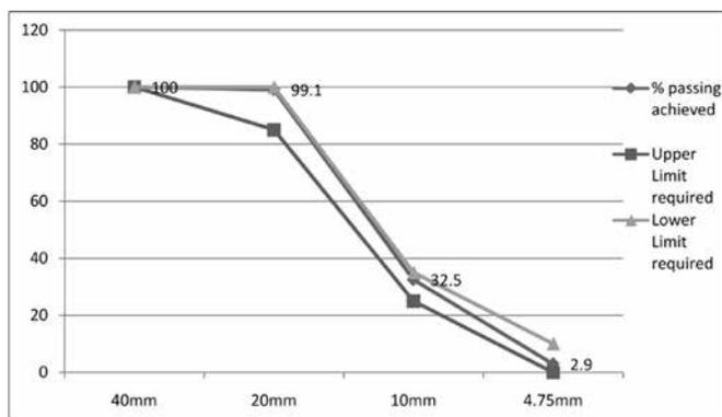
**Fig. 6. Particle Size Sieve Analysis (Coarse Aggregate – 20mm nominal size) (a) Fresh Aggregate**
