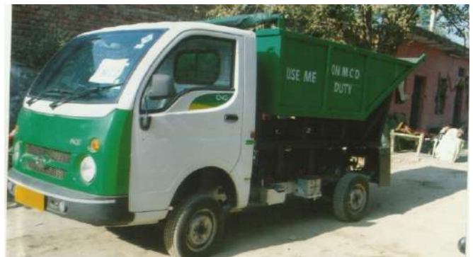
Fig: 1: Auto Tipper for Door-to-Door Waste Collection
