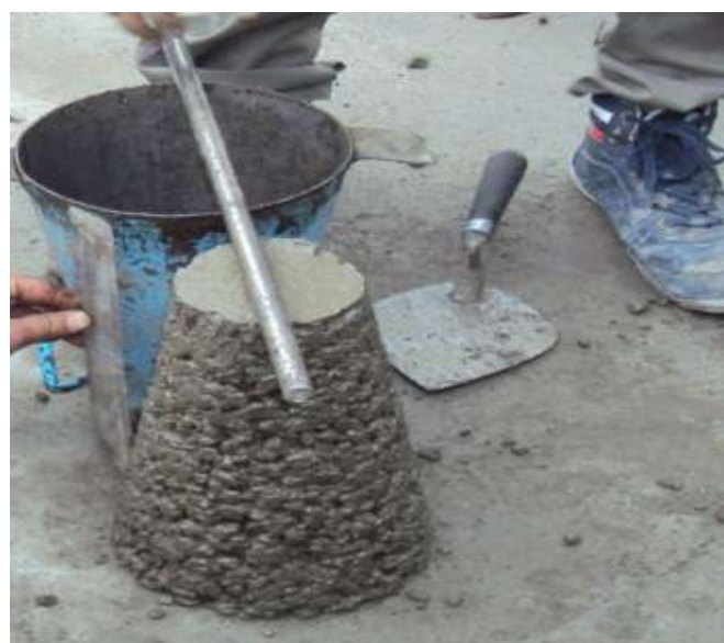
Slump Test for OPC and RA
