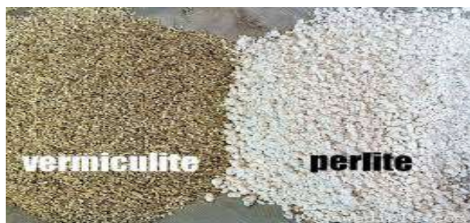
Fig. 5: LW Perlite and Vermiculite
