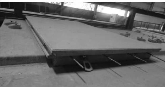
Fig. 10: Precast Wall Panels (1400 Sqm/day)
