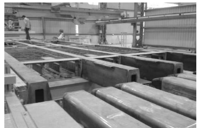
Fig. 12: Precast Column Casting (130 Columns /Day)
