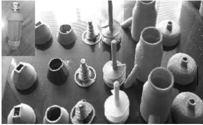
Fig. 6a : Parts of Extruder Units so Printed in PLA
