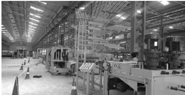
Fig. 9: Lattice Girder Manufacturing Facility for Precast Slabs (7500 m 2 /day)
