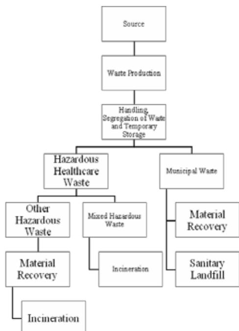
**Fig. 1: Flow Diagram of Bio Medical Waste Management**
