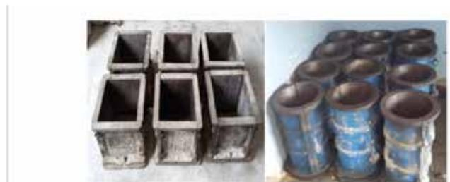
**Fig. 7: Cube and Cylinder Moulds**
