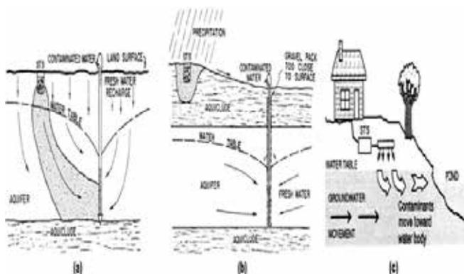
**Fig. 3: Contamination of Sub-surface (a, b) and Surface (c) Water Sources by a Failing STS**
