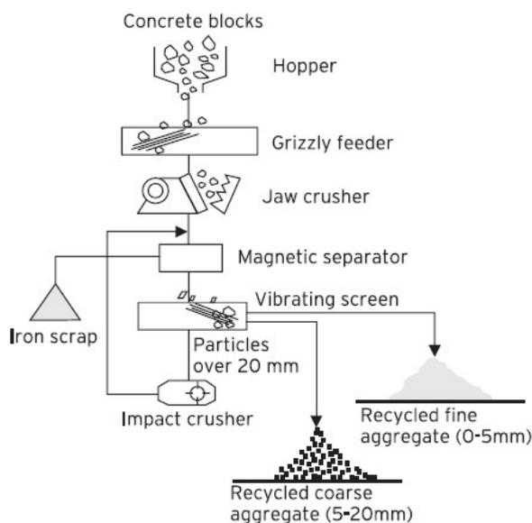
**Fig.2: Processing of Concrete Waste into Aggregate**
