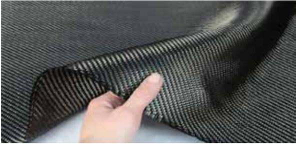
**Fig. 9: Carbon Fibre Fabric**
