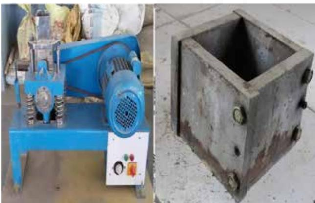
**Fig. 4: Vibrator and Compression Strength Mould**
