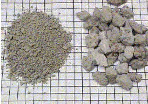
**Fig. 3: Blast Furnace Slag**
