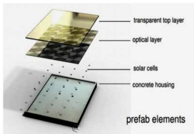
**Fig.4: Components of Solar Roadway**
