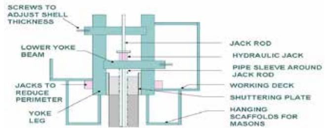
**Fig.25: Slip Forming Equipment**
