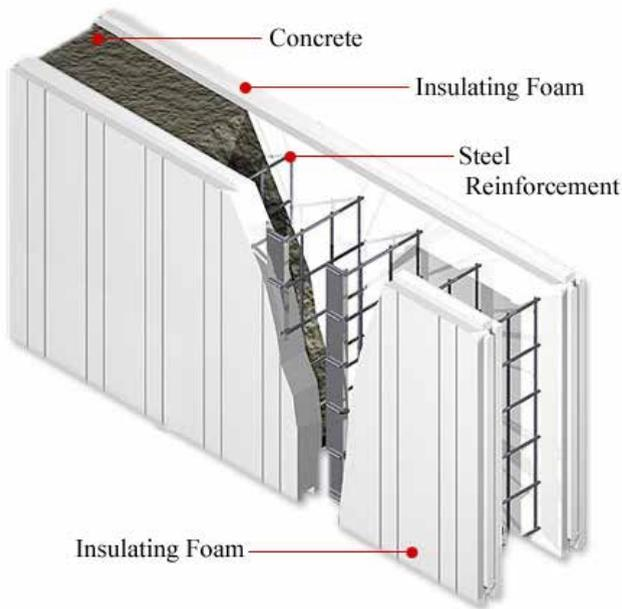
**Fig. 3: Insulating Concrete Forms Installation**
