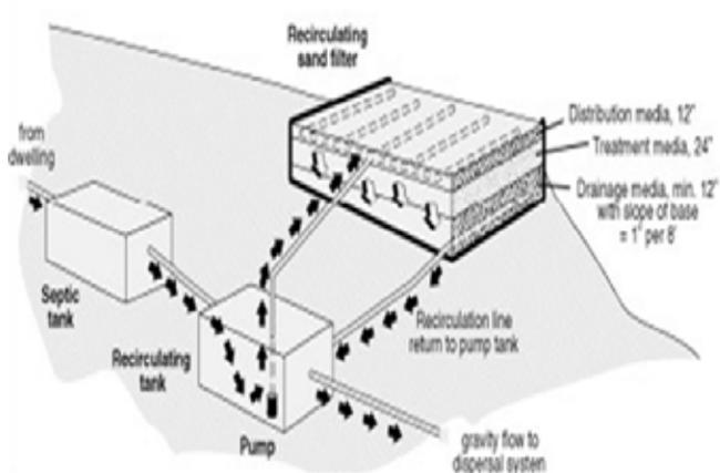
**Fig. 5: Specific System Design Using a Re-circulating Sand Filter**
