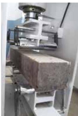
**Fig.14: Setup for Flexural Strength Test**
