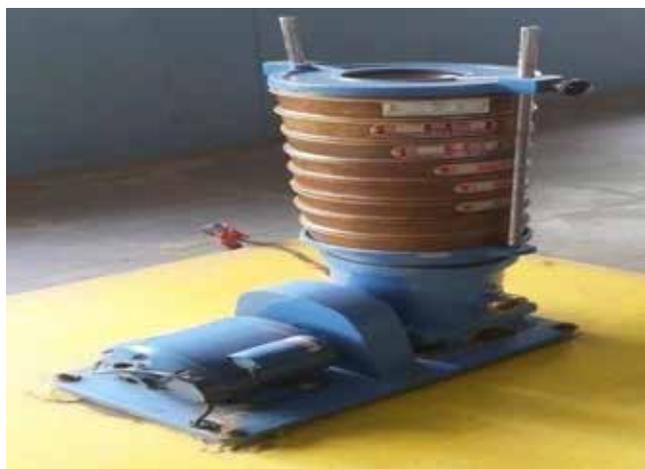
**Fig.6: Set of Sieves with Sieves Shaker**
