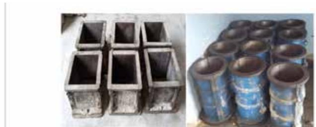
**Fig. 7: Cube and Cylinder Moulds**
