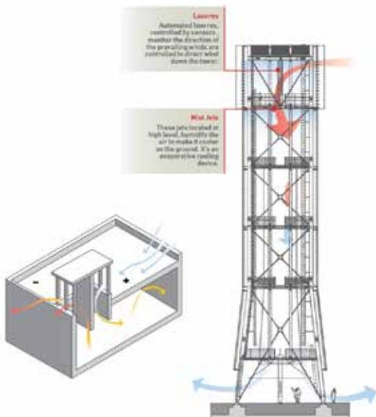
**Fig.2: Operation mechanism of modern wind tower (right), compared to traditional wind tower (left).**
