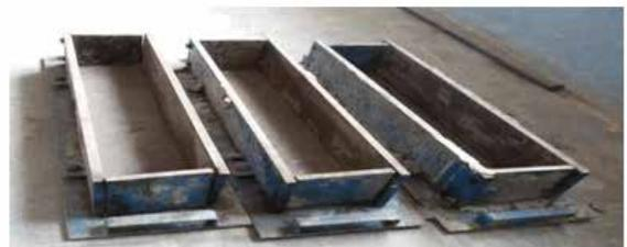
**Fig. 8: Beam Mould**
