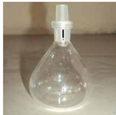
**Fig. 3: Specific Gravity Bottle**
