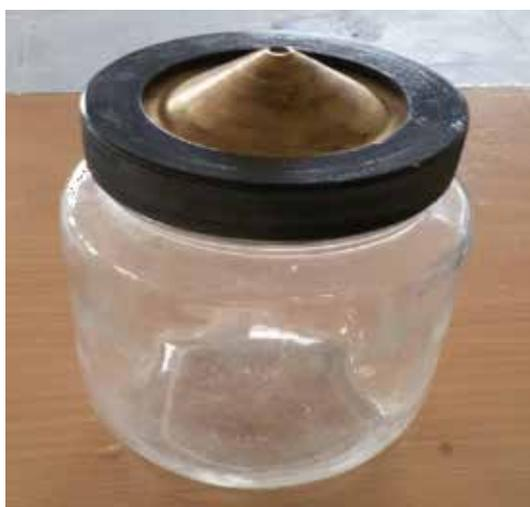
**Fig.7: Specific Gravity Bottle for Aggregates**
