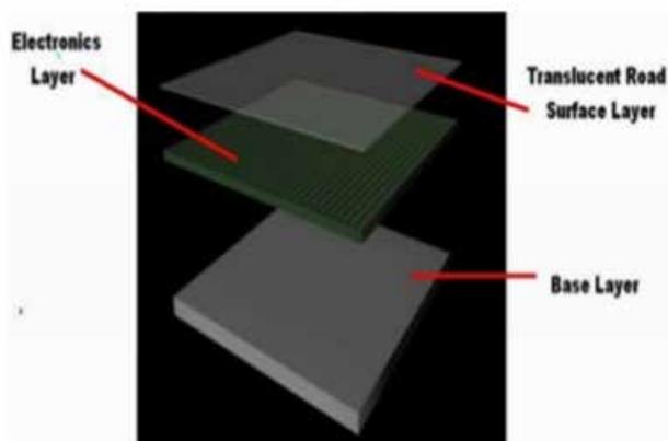
**Fig. 3: Structure of Solar Roadways**
