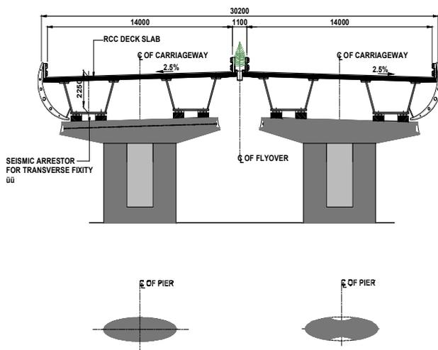
**Fig. 20: Composite Steel Box Girder for Main Flyover**
