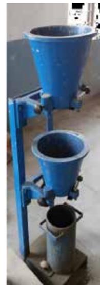
**Fig. 12: Apparatus for Compaction Factor Test**
