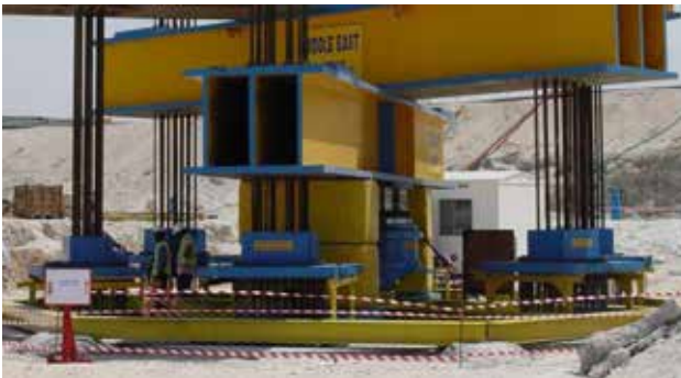
Enhanced pile load tests using Osterberg Cells
