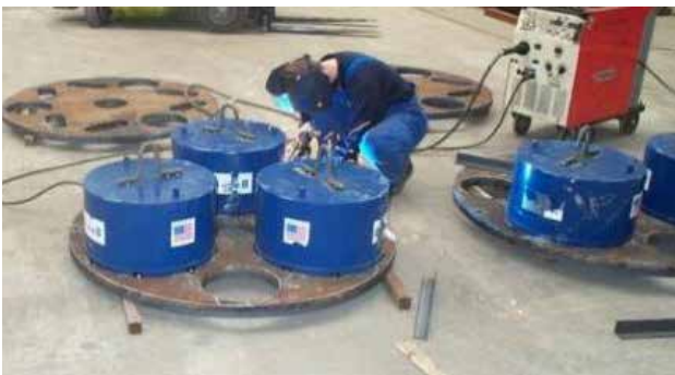
Enhanced pile load tests using Osterberg Cells
